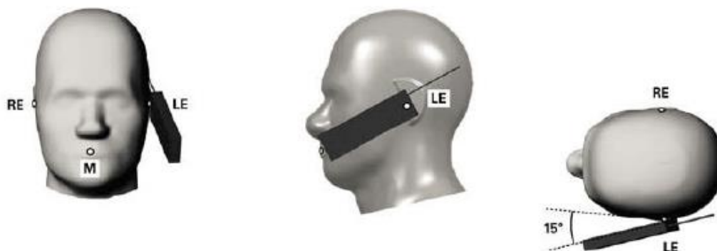
Fig.11.4 Illustration for Tilted Position
