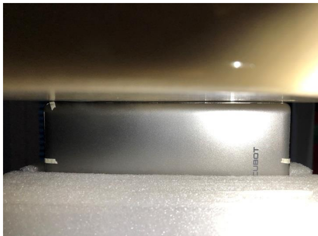
Limb – Left (Test distance: 0mm, Thickness of DUT: 9mm)
