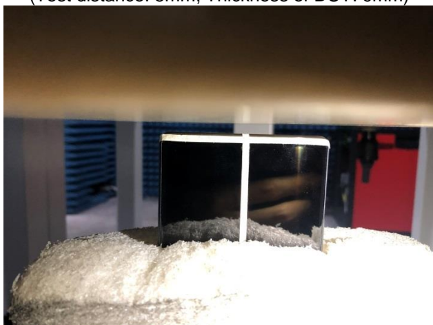
Body worn – Top (Test distance: 5mm, Thickness of DUT: 9mm)
