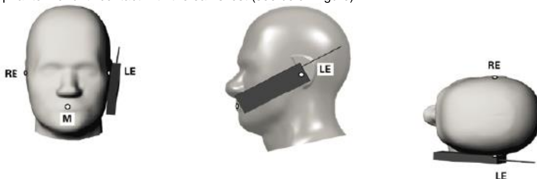
Fig. 11.3 Illustration for Cheek Position
